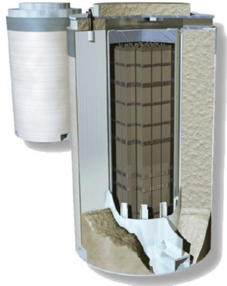
Dry casks have thick shielding to protect workers and the public from radiation
